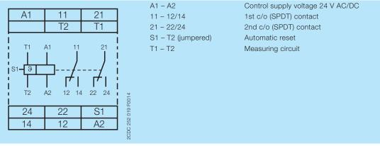
Connection diagram CM-MSS.32
