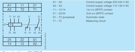
Connection diagram CM-MSS.33
